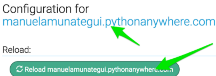
Figure 5-22. The big green reload button to update the web server after any changes
